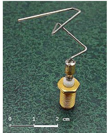
The 2006 NASA ST5 spacecraft antenna. This complicated shape was found by an evolutionary computer design program to create the best radiation pattern. It is known as an evolved antenna .
